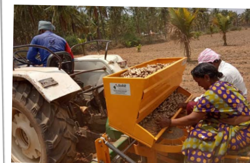
The semi-automatic Potato planter developed by the GIC project in cooperation with Rohit Krishi Industries Pvt. Ltd.
